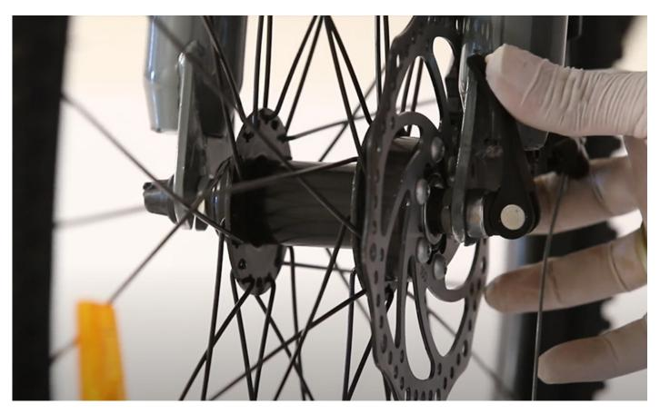
STEP 8-9: Fix the Front Wheel and Quick Release mechanism
