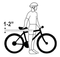
THE SEAT POST "MINIMUM INSERTION" / "MAXIMUM HEIGHT" MARK SHOULD NOT BE VISIBLE WHEN THE SEAT POST IS INSERTED INTO THE SEAT MAST OF THE BIKE. DO NOT RAISE THE SEAT POST BEYOND THIS MARK. THE SEAT POST OR FRAME MAY BREAK CAUSING YOU TO LOSE CONTROL AND FALL. ALWAYS CHECK TO MAKE SURE THE SEAT POST ADJUSTING MECHANISM IS TIGHTENED SECURELY BEFORE RIDING.
