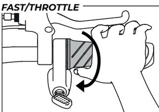
Make sure PAS is more than 0. Rotate the half throttle on the right handlebar grip.
