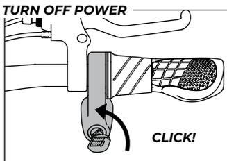
Alternatively, rotate key counter clockwise to turn off bike.
