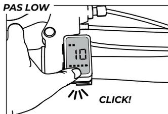
Once display is on, increase or decrease pedal assistance as per need, from 1 to 5. If you stop pedalling, the motor assist will stop
