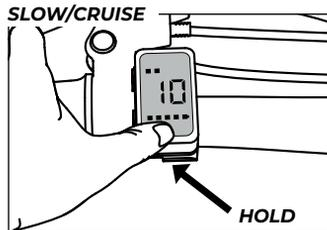
Press and hold the bottom part of display button to cruise at a constant speed
